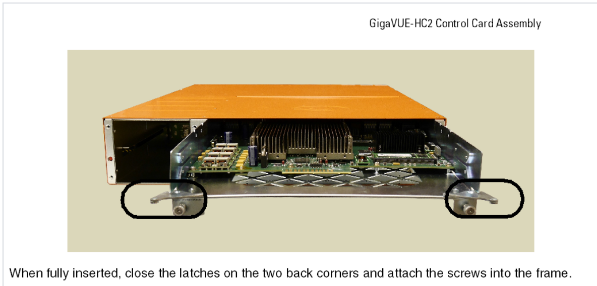
Figure 10: Installing Control Card to the rear of the GigaVUE-HC2
